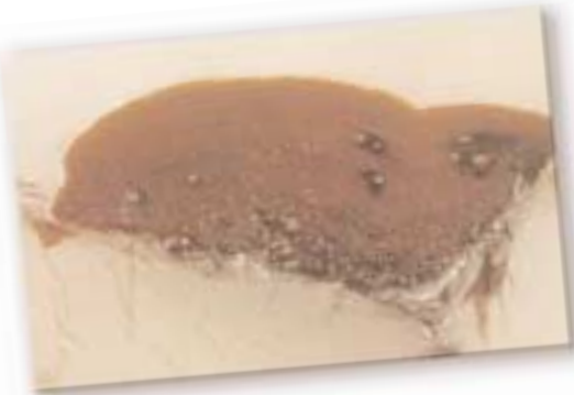
Dry Rot fungus is the cause of major decay in timber. A durable stone presents no problem similar to this.
