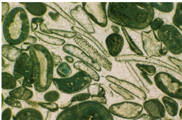
Fig. 6 Typical texture of Bath Stone seen in thin-section. Ooliths and shell fragments touch at point contacts; intergranular and secondary macroporosity are completely filled by calcite spar. This example is Box Ground Stone, which has well-developed layers of shell debris.
