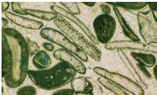
Fig. 12a Effects of large calcite cement crystals growing across grain boundaries. a , the edges of formerly aragonite shell fragments are usually represented by microporous lines of weakness where lines of small seed crystals run along the junction of the primary and the secondary (biomouldic) porosity (the micrite envelope). b , if some crushing took place after the aragonite dissolution but before the start of spar growth, then the micrite envelopes became broken and discontinuous. This allowed a stronger fabric of larger calcite crystals to cross through the gaps from primary to secondary porosity and hence interrupt the weak zone that run along the edges of the grains. This fabric is often seen in the shellier Lincs Limestone and Inferior Oolite freestones.
