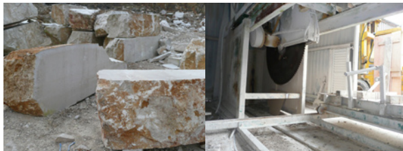
Fig. 32 1.Primary saw and sawn block at Brassington Moor Quarry (© Longcliffe Quarries Ltd 2007).
