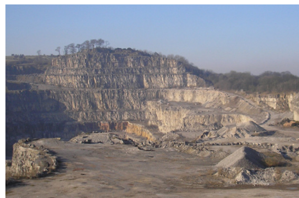
Fig. 30 Overview of Middle Peak Quarry. The 1980s extraction of Hopton Wood took place on the bench to the right, just below the low boundary face. Immediately beyond was Wheatcroft's/Hopton Wood Stone Co's c19th Middlepeak (roadside) operation. (Author)
