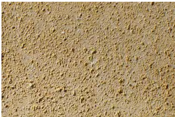
Fig. 13 Close-up of freshly cut surface of Dundry Stone, which is non-oolitic and largely composed of bioclasts. The small holes represent primary and secondary (biomouldic) macroporosity that are incompletely filled by calcite cement.
