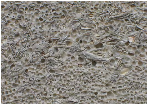
Fig. 7 Weathered surface of a spar-prominent stone in which the microporous ooliths have weathered out to leave the shell fragments and the encasing calcite cement conspicuously exposed.
